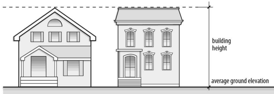
Figure 90-20: Building Height Measurement
